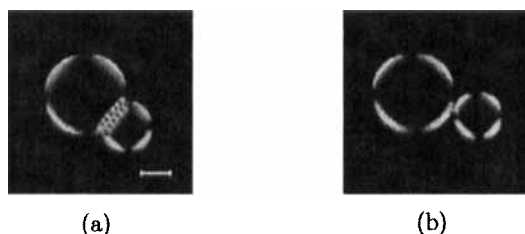
FIGURE 3 Equilibrium Sm-A domains in an I phase at 36.0°C observed with the analyzer and polarizer crossed ( L = 5\mu\text{m} ) before (a) and after electric-field ( 2.0\text{V}/\mu\text{m} ) application (b). The bar indicates 20\mu\text{m} .
